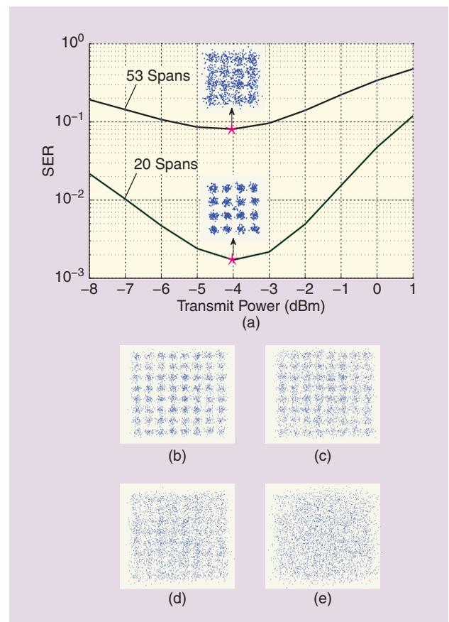
**[FIG2]** (a) The SERs of a nonlinear fiber-optic link with 20 and 53 spans together with the scatter plots of the received signals for a 16-QAM at the minimum SER, marked by two stars. The scatter plot of the received signal for a nonlinear fiber-optic link with 64-QAM operating (b) 6.5, (c) 4.5, (d) 2.5, and (e) 0 dB away from the AWGN channel capacity at a spectral efficiency of 5.5 bits per polarization. The values of the system parameters are given in Table 1.
