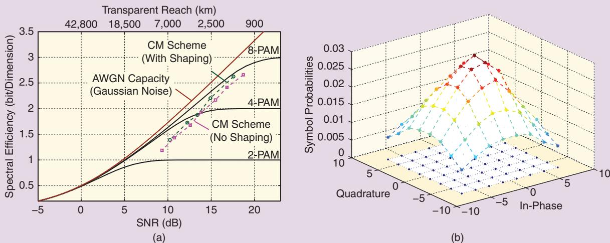
**[FIG7]** (a) The spectral efficiency per dimension versus the transparent reach and the SNR for a non-DM link with EDC. The CM scheme curves are based on the results given in [16] and the spectral efficiency for the Gaussian noise model is computed by  $\log_2(1 + \text{SNR})/2$ , where  $\text{SNR} = |\zeta|^2 P/\sigma^2$ . (b) The 2-D symbol probabilities of the probabilistically shaped 4-D CM scheme.
