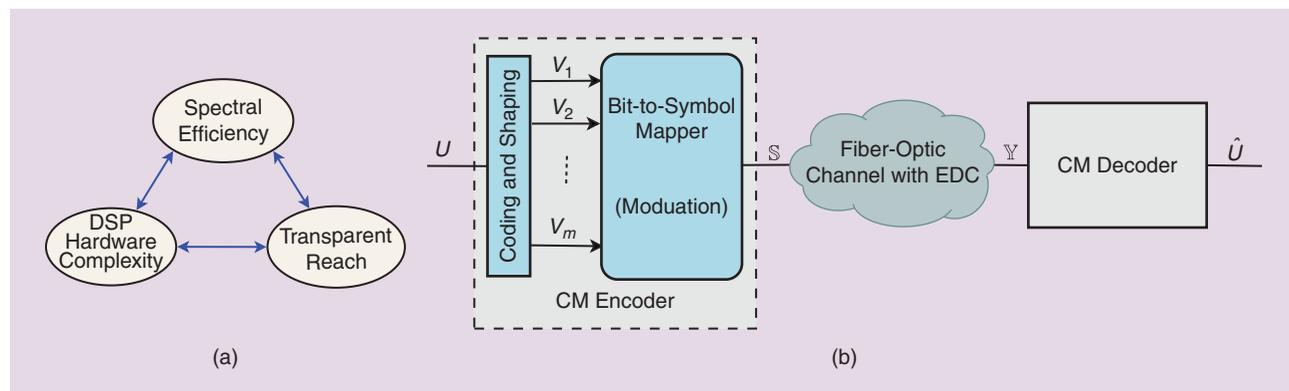
**[FIG1]** (a) The three main factors in the design of a CM scheme for fiber-optic links. (b) A fiber-optic link including a CM encoder and decoder with EDC ( $U$  and  $\hat{U}$  are the transmitted and decoded information bit sequences, respectively).
