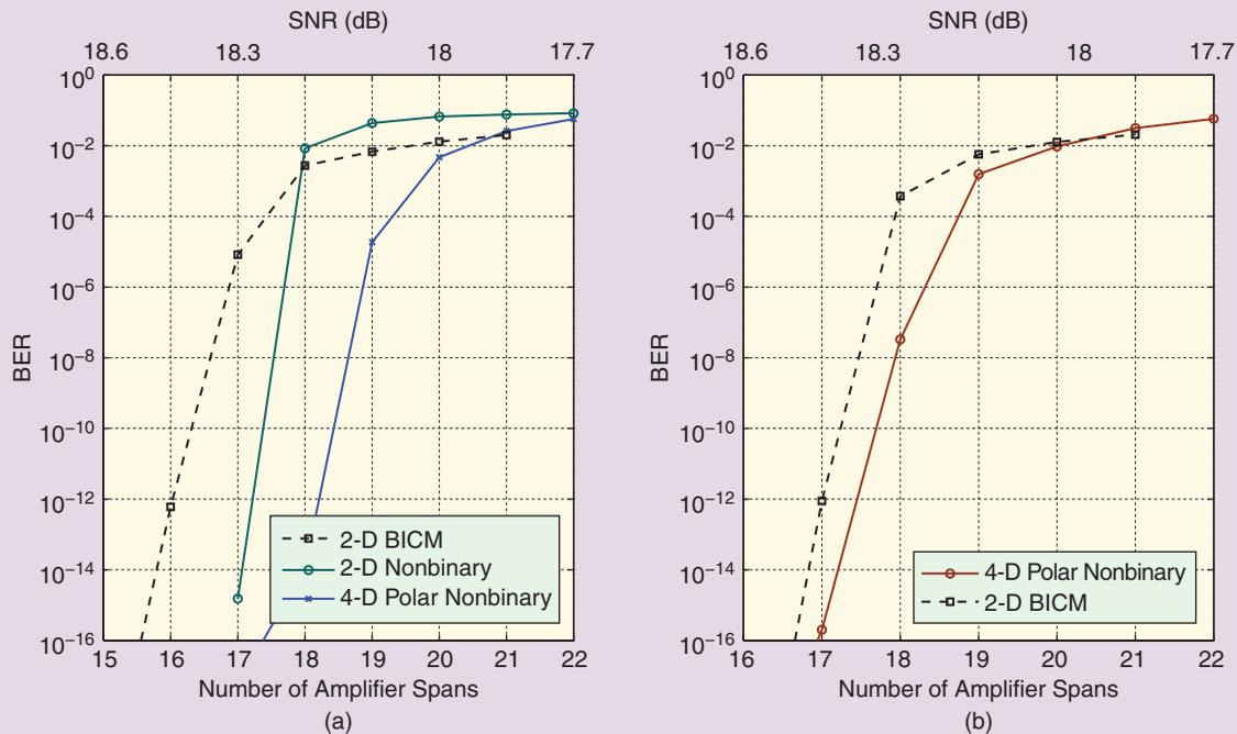
**[FIG6]** (a) The BER of three CM schemes with information-block-length-constraint. (b) The BER of 2-D and 4-D CM schemes with binary and nonbinary LDPC codes, respectively, and similar complexity. All the CM schemes use PM 64-QAM with 21% coding overhead and have therefore the same spectral efficiency.
